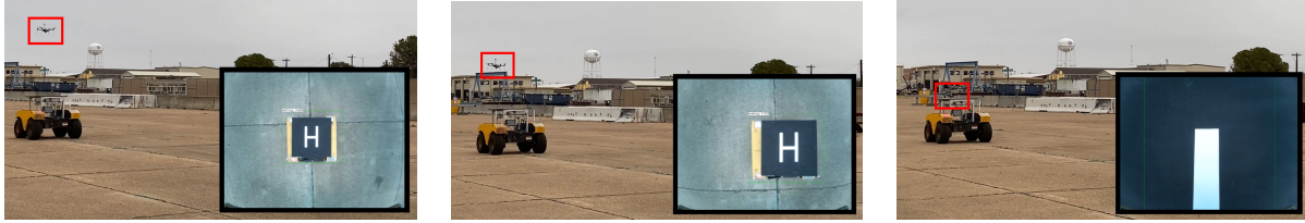
Figure 4.24: Visual time series of a landing experiment with the Warthog UGV. The UAS is marked by the red box.
