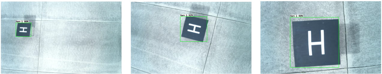
Figure 2.12: Examples of cart landing target detection.
