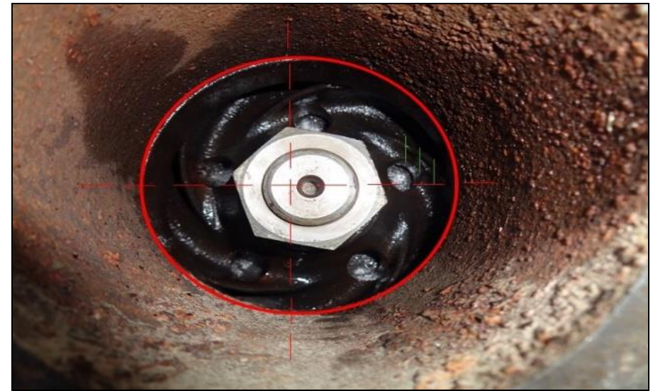
View from Inlet of the Pump: Impeller eye and Nozzle are not concentric
