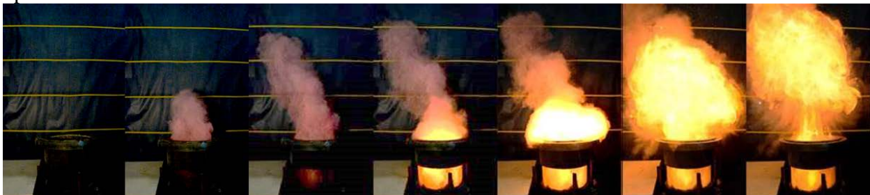
Figure 2. Representative still shots from a video taken of a deflagration of an organic dust. The dust is first injected, a spark at the center of the chamber ignites the dust, and then the flame propagates out of the chamber and through the dust cloud. Yellow lines behind the system are spaced at one foot intervals.
