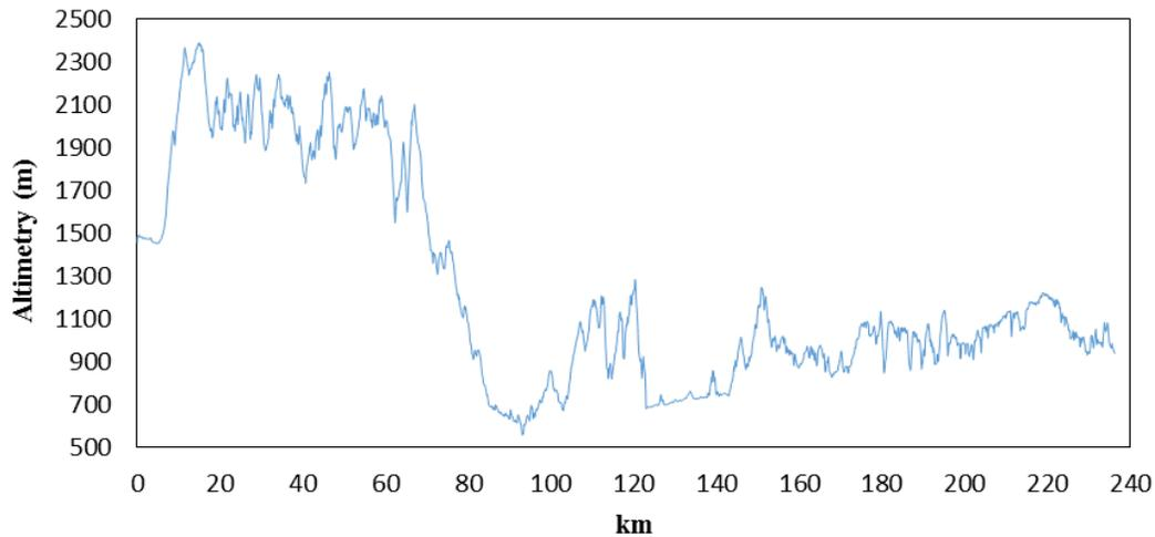
**Figure 8. Altimetry profile of the pipeline**
