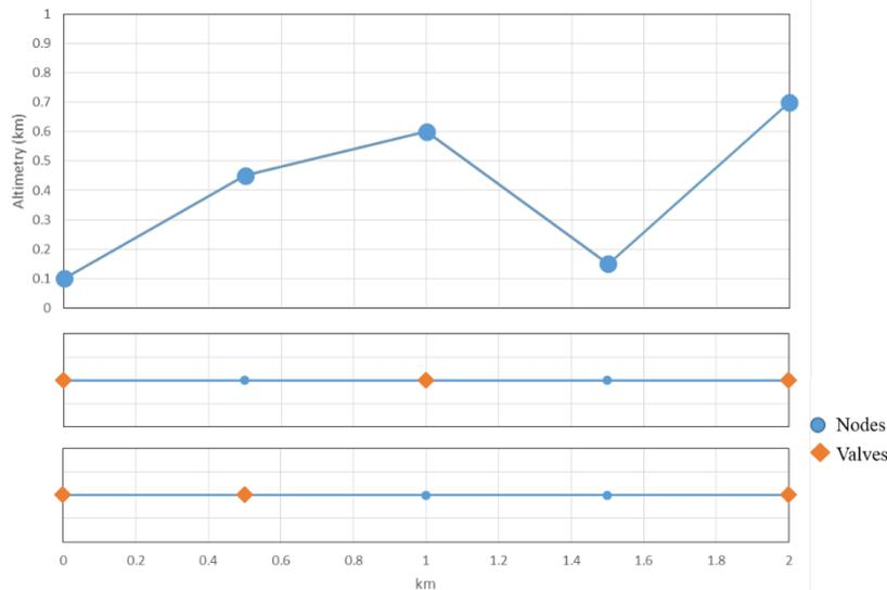
**Figure 1. Illustration of a linear pipeline segment with connection points (nodes) each 500 m. Two different configurations of valve location are presented.**
