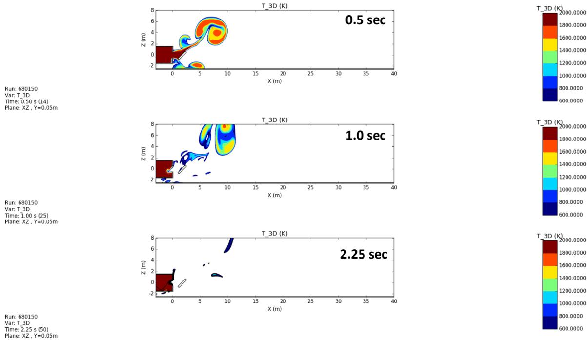
Figure 4. Time sequence of fireball temperature contours showing FLACS simulation of a propane/air ( $\Phi = 1$ ) vented explosion for a  $3\text{ m} \times 3\text{ m} \times 3\text{ m}$  enclosure with a  $1\text{ m}^2$  vent that
