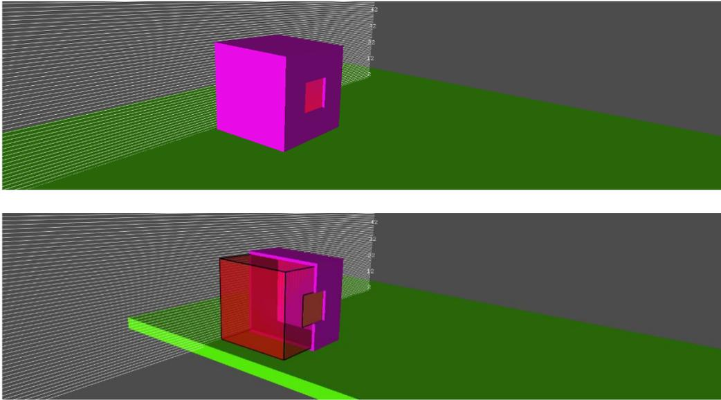
*Figure 1. Sample CFD Model geometry without a deflector plate. The top image shows the entire geometry, while the bottom image shows a cut view highlighting the flammable cloud and explosion vent area.*
