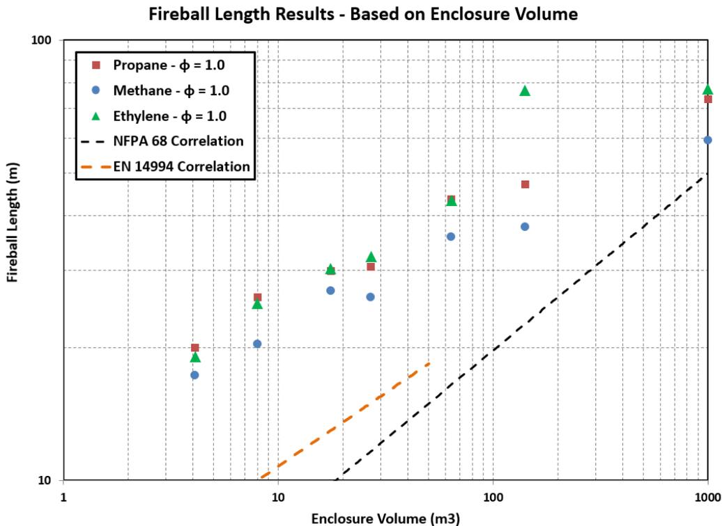
Figure 5: FLACS calculated fireball length for propane/air, methane/air, and ethylene/air mixtures at an equivalence ratio of 1 compared to the NFPA 68 and EN 14994 predicted values.
