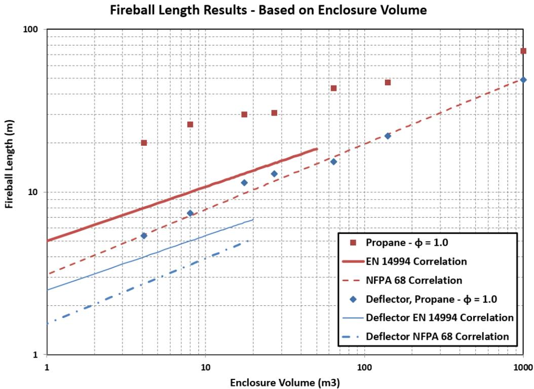
Figure 6. FLACS calculated fireball length for propane/air mixtures with and without a deflector plate as a function of enclosure volume compared to the NFPA 68 and EN 14994 predicted values.
