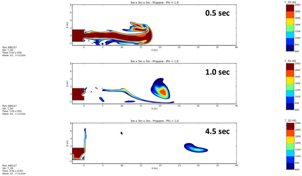
Figure 3. Time sequence of fireball temperature contours showing FLACS simulation of a propane/air ( $\Phi = 1$ ) vented explosion for a  $3\text{ m} \times 3\text{ m} \times 3\text{ m}$  enclosure with a  $1\text{ m}^2$  vent that activates at 0.1 barg. The maximum overpressure ( $P_{red}$ ) for this scenario is 0.33 barg; and the maximum fireball extent is calculated to be 31.8 meters, based on the 1,000 K contour.
