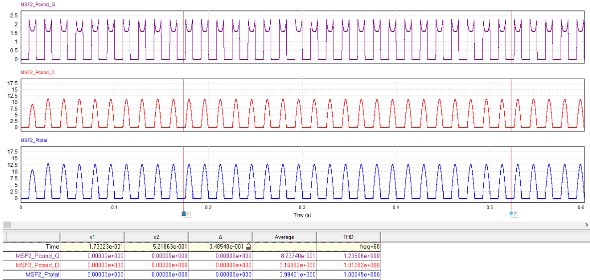
Figure 39. Conduction and Switching Losses for MOSFET1
