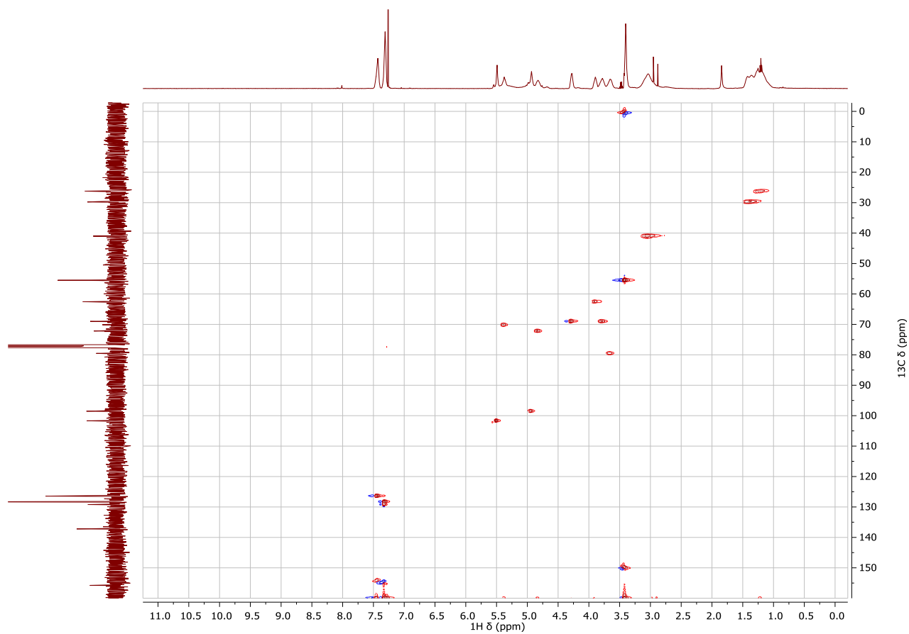
Figure A-75. ^1\text{H} - ^{13}\text{C} HMQC (500 MHz-125 MHz, \text{CDCl}_3 ) spectrum of 7a in \text{CDCl}_3 , nt = 32, ni = 200.
