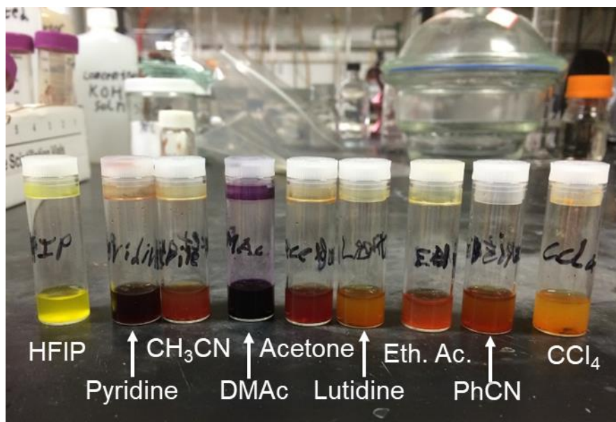
Figure 5-7. Oligomer 26 shows remarkable solvatochromic effect as a suspension in various solvents.
