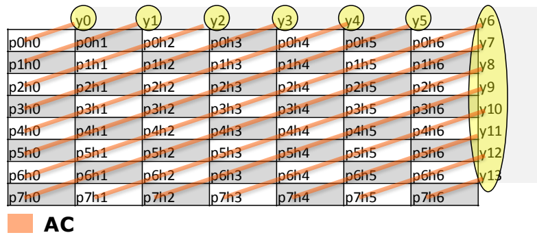
(b) Diagonal accumulation in the 16-bit FIR filter operation
