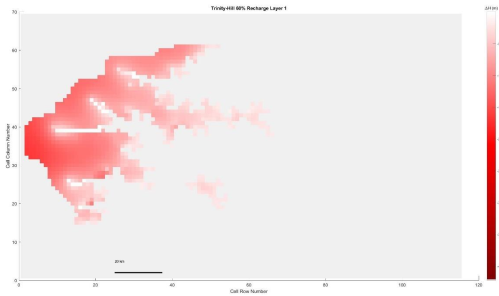
Figure 5. 524 Trinity Hill, 60% original recharge hydraulic head spatial distribution of layer 1
