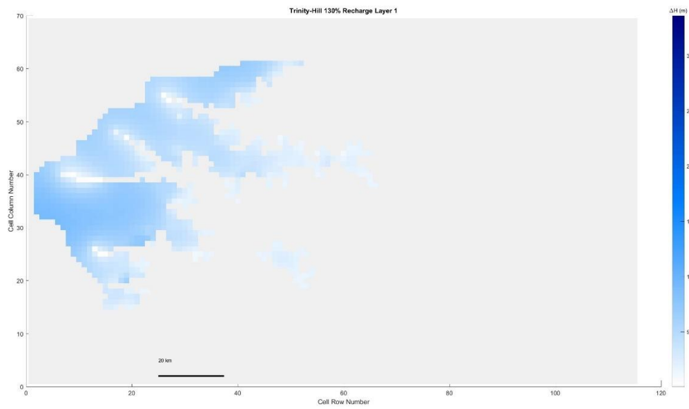
Figure 5. 518 Trinity Hill, 130% original recharge hydraulic head spatial distribution of layer 1
