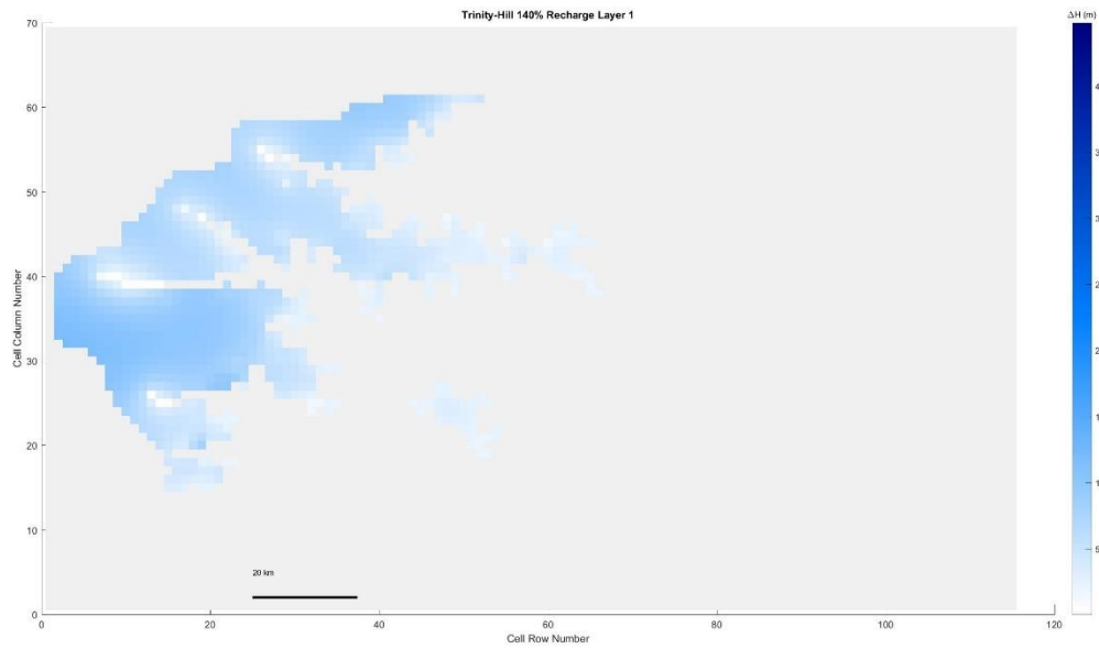
Figure 5. 517 Trinity Hill, 140% original recharge hydraulic head spatial distribution of layer 1
