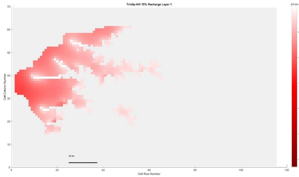
Figure 5. 523 Trinity Hill, 70% original recharge hydraulic head spatial distribution of layer 1
