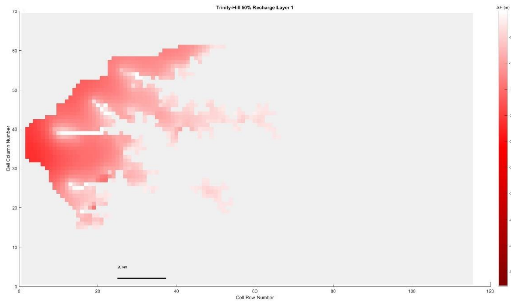
Figure 5. 525 Trinity Hill, 50% original recharge hydraulic head spatial distribution of layer 1
