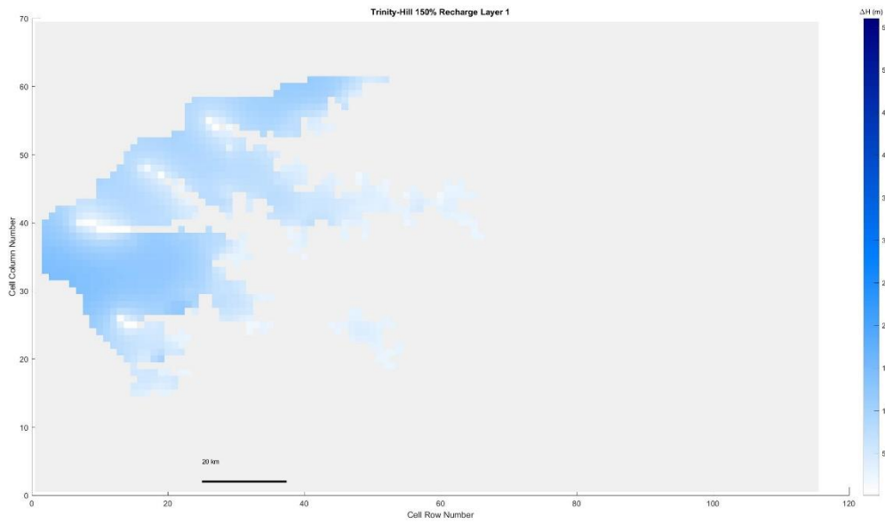
Figure 5. 516 Trinity Hill, 150% original recharge hydraulic head spatial distribution of layer 1
