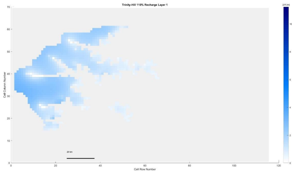
Figure 5. 520 Trinity Hill, 110% original recharge hydraulic head spatial distribution of layer 1
