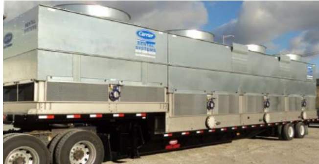
Figure 5-15: 1000-Ton Commercial Cooling Tower, reprinted from [56]
