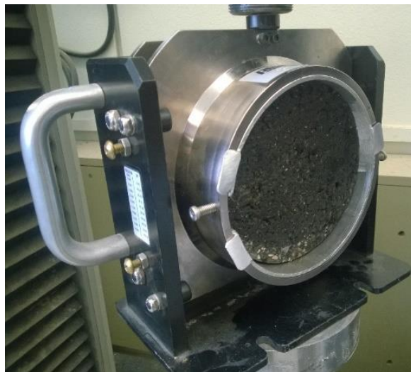
Figure 11 Test apparatus of direct shear test.
