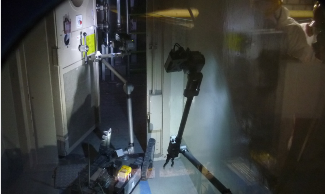
Figure 1.1: Two iRobot Packbots Working Together to Open a Door during the Fukushima Daiichi Nuclear Accident (Image Courtesy: JAEA)
