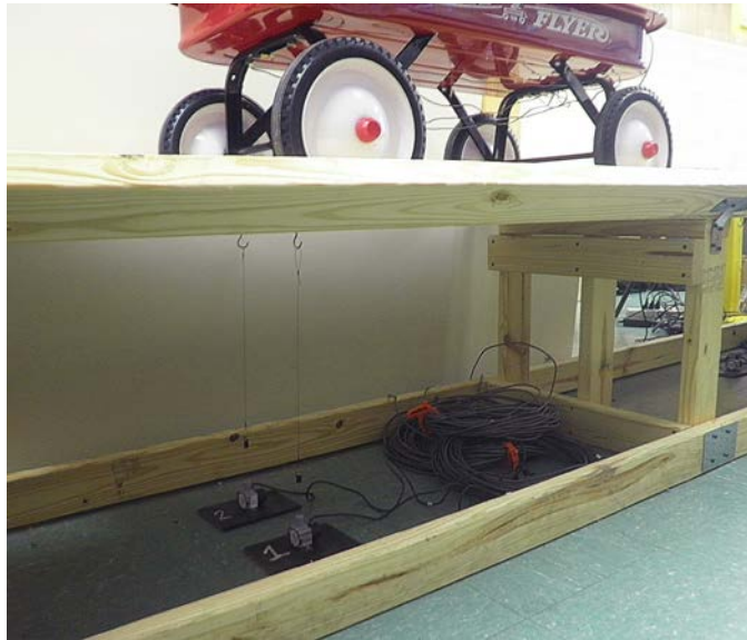
Figure 2.17: String Potentiometer Installation on Small-Scale Bridge
