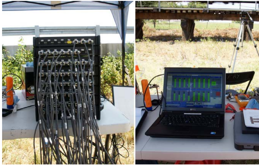
Figure 2.27: Bridge 17.14 Data Acquisition System
