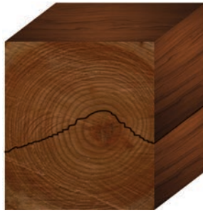
Figure 1.3: Split Stringer Caused by Shear Cracking
