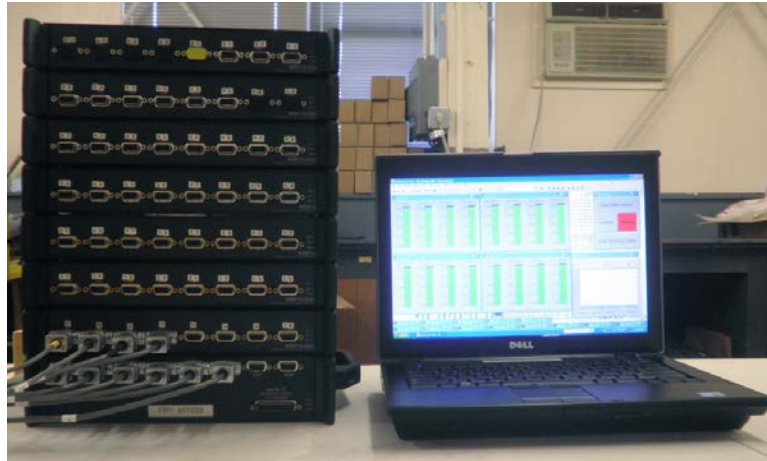
Figure 2.18: Small-Scale Experiment Data Acquisition System
