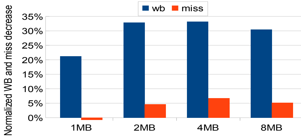
Figure 2.13: Normalized writebacks and misses decrease under varied cache sizes, SPEC2006 (higher is better).
