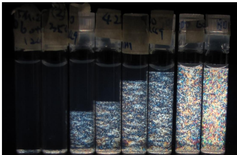
Figure 22. ZrP nanodisks suspensions with increasing concentrations from left to right observed between crossed polarizers. Volume fraction of the nanodisks from left to right: 0.38%, 0.44%, 0.50%, 0.53%, 0.56%, 0.63%, 0.75% and 1% respectively. The colorful portions indicate nematic ordering of disks. Due to gravity, nematic tactoids settle at the bottom. This picture is taken after 3 days of gravity sedimentation of nematic tactoids.
