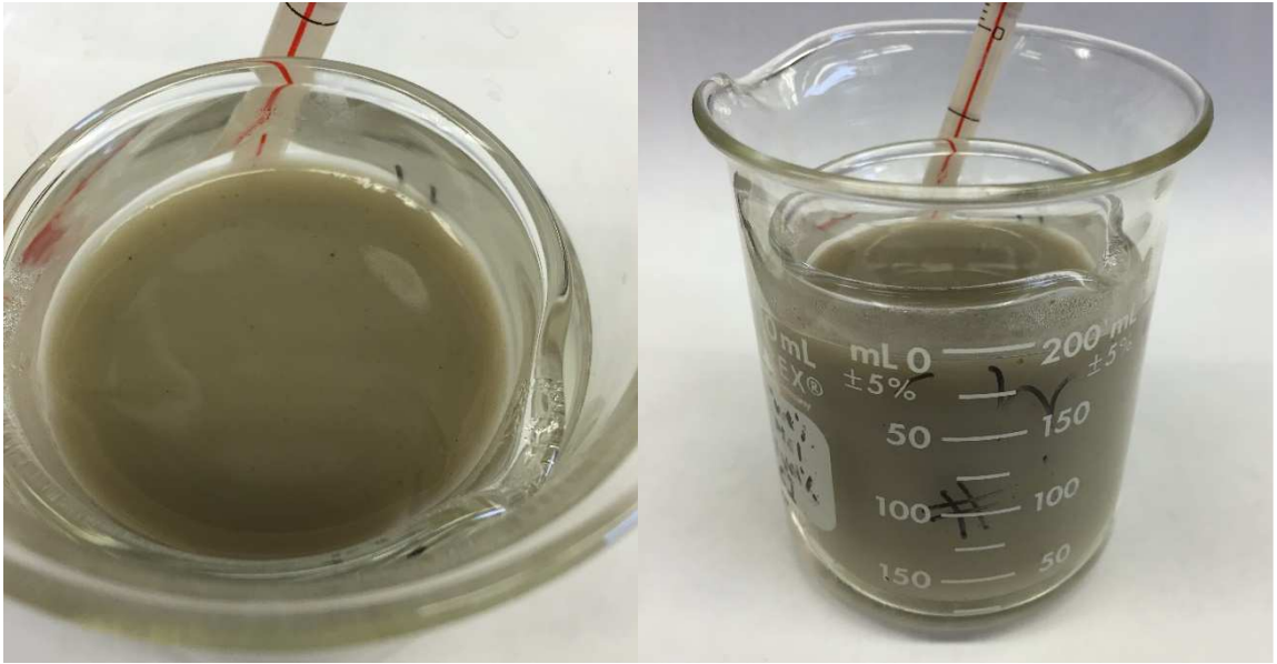
Fig. A- 1—Base Fluid in a water bath at 212°F (100°C) at time zero.
