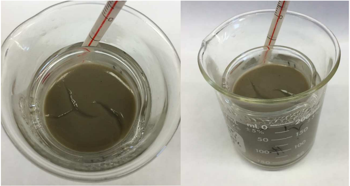
Fig. A- 3—Base Fluid in a water bath at 212°F (100°C) after 60 minutes.
