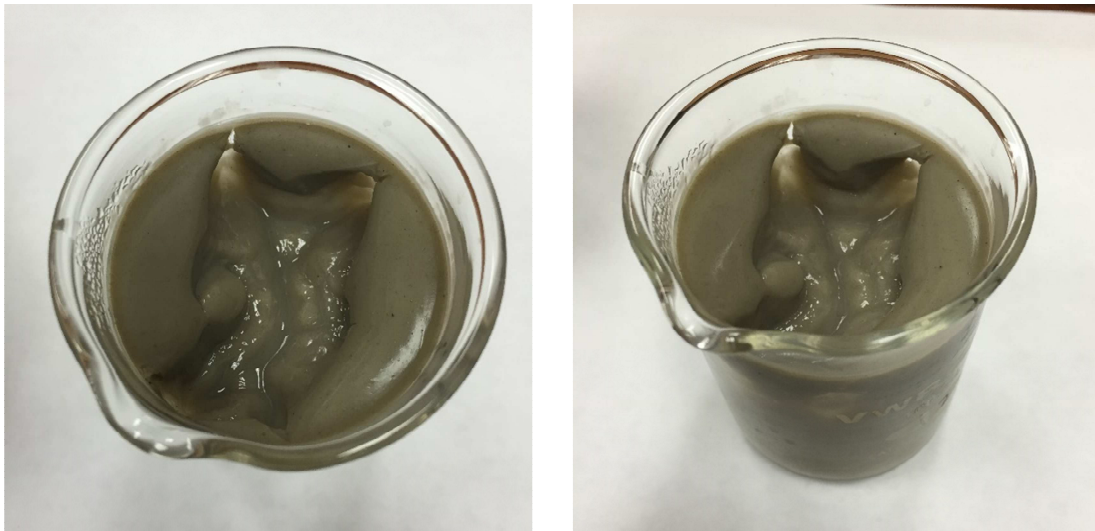
Fig. A- 7—Base Fluid left for 16 hours after thermal aging in a water bath at 212°F (100°C) for 150 minutes.
