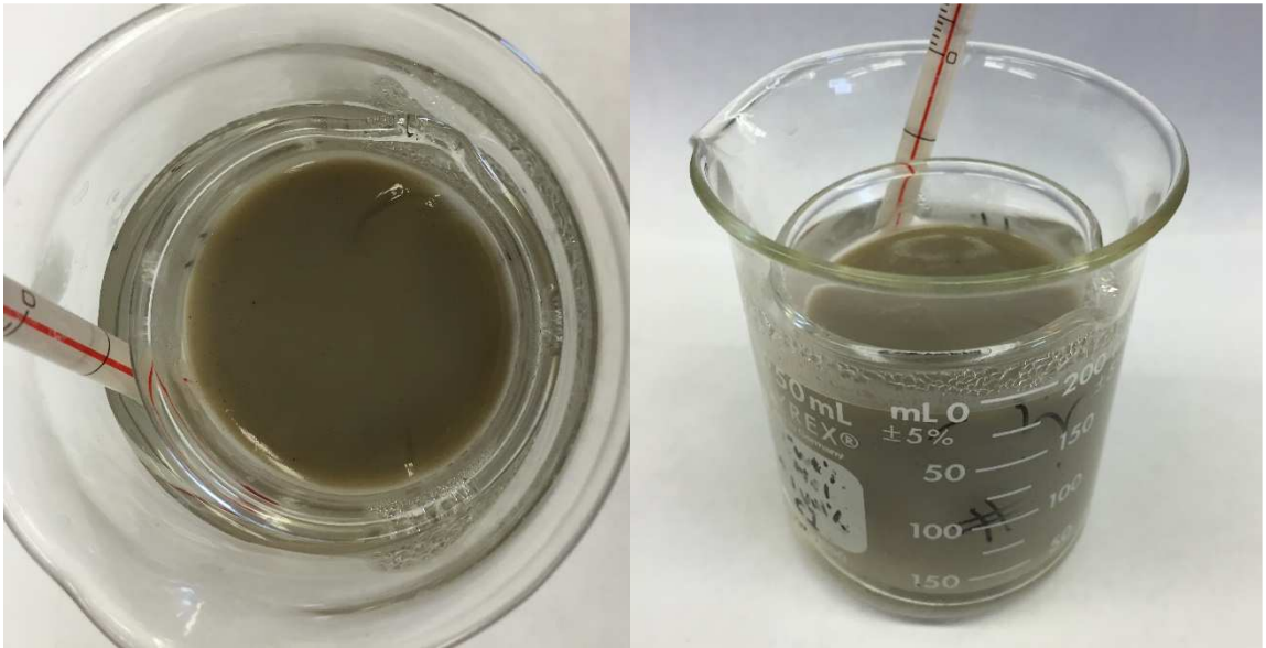
Fig. A- 2—Base Fluid in a water bath at 212°F (100°C) after 30 minutes.
