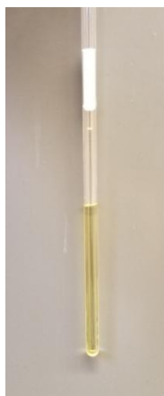
Figure 6.2. Capillary insert with ClPPh 2 centered inside a 5 mm NMR tube.
