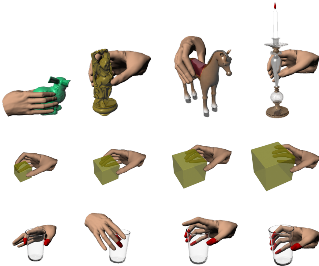
Figure III.7: Object grasping: (top) grasping objects of different shapes; (middle) grasping a cube of different sizes; (bottom) grasping a cup with different grip modes; from left to right: thumb and index finger, thumb and middle finger, all fingers except index fingers, and all fingers.
