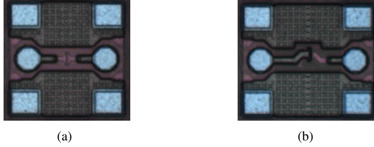
Figure 2.10: Micrographs of 12 \times 32 \times 1\mu\text{m}/28\text{nm} transistor test structures used in power capability verification: (a) L_{deg} = 0 , (b) L_{deg}=14\text{pH} single-ended. Reprinted from [1].
