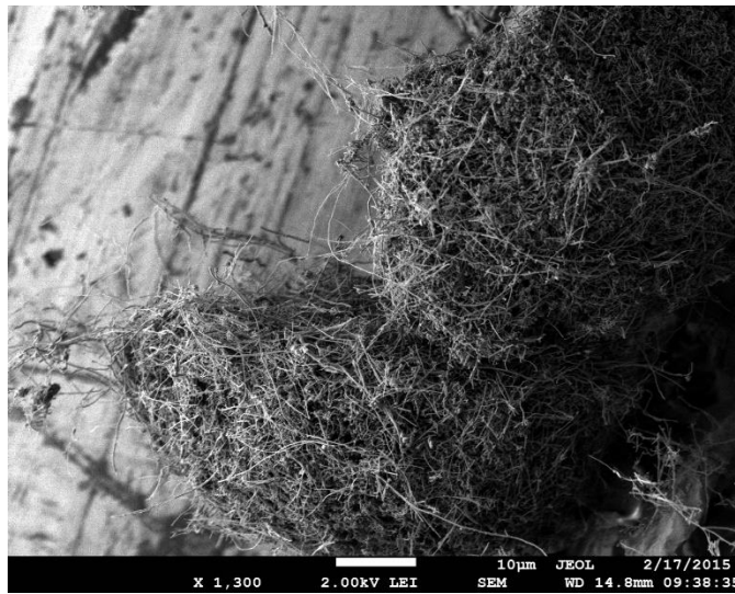
Figure 16: CNF tangled hairball structure as received from Pyrograf Products. This tangled structure is why sonication (or other effective means of dispersion) is required.
