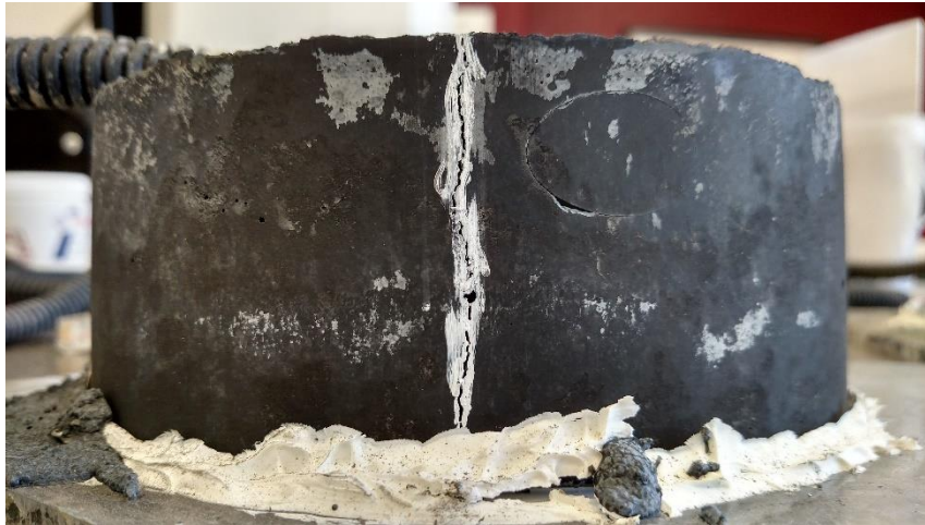
Figure 72: Hybrid microfine cement mortar ring with 2wt% CNFs with a macrocrack (highlighted in white paint).
