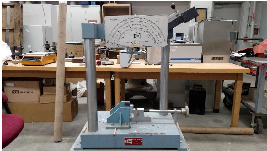
Figure 55: Izod impact test equipment.
