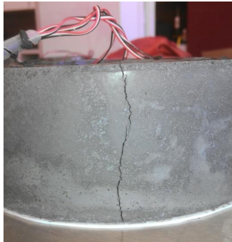
Figure 67: OPC restrained mortar ring with 0.1wt% CNFs and a macrocrack.
