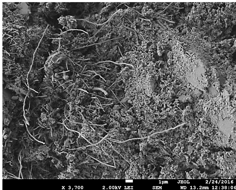
Figure 89: 2wt% CNFs hybrid OPC hydrated showing CNFs.
