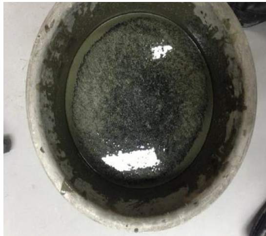
Figure 24: CNFs in fresh cement paste showing that uniform dispersion was not achieved. The black specs in the paste are agglomerations of CNFs.
