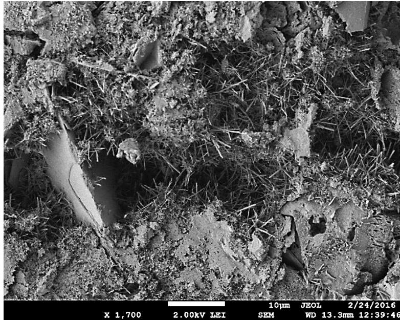
Figure 90: 2wt% CNFs hybrid OPC hydrated showing CNFs and ettringite in a large crack. CNFs and ettringite are nearly indistinguishable at this magnification.
