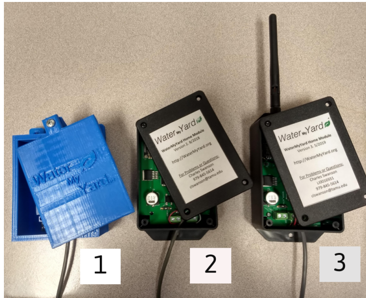
Figure 3.7: The progressions of the WMY module through versions 1, 2 and 3. Version 1 was built using off-the-shelf components. We designed a PCB for Version 2. The design was further refined for Version 3 of the WMY module
