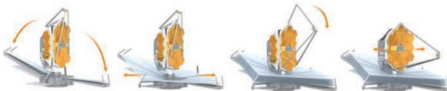
Figure 2.39 Deployment process of the James Webb telescope [23].
