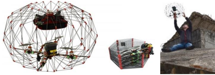
Figure 2.18 (left) Expanded cargo delivery system containing first aid kit, (middle) Collapsed cargo delivery system, (right) User safely catching drone [45].
