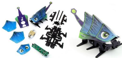
Figure 2.41 Components used to create a fully assembled Kamigami Robot [82].
