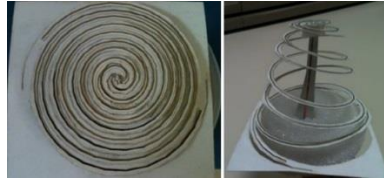
Figure 2.38 Spiral antenna in flat and expanded configurations [78].
