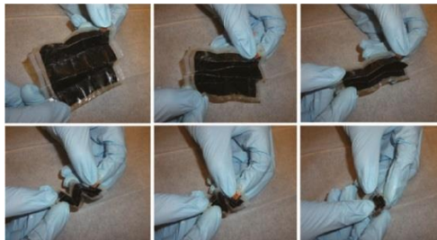
Figure 2.5 Folding lithium-ion battery using Miura-ori crease pattern [7].
