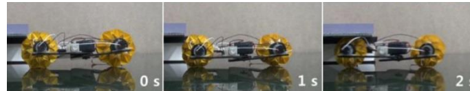
Figure 2.10 Robot quickly navigating obstacles using deformable origami wheel [31].
