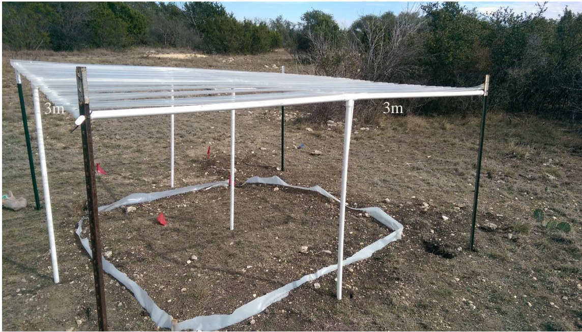
Figure 3. Rainout shelter (3 x 3m) in field
