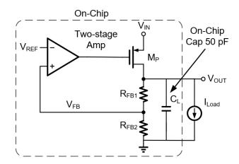
Figure 3.2: Macro model of the uncompensated LDO
