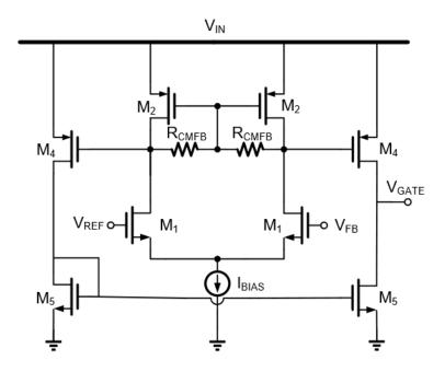
Figure 3.8: Two-stage error amplifier schematic
