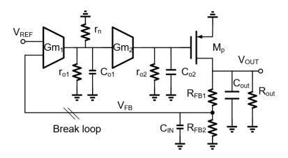
Figure 3.22: AC open-loop simulation circuit
