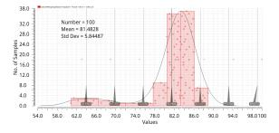
Figure 4.16: Phase margin for 100 mA load
