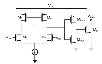
Figure 3.16: Analog comparator
