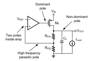
Figure 3.18: Capacitor-less LDO poles location
