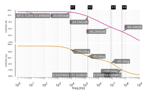
Figure 3.27: Frequency response for 0 A load
