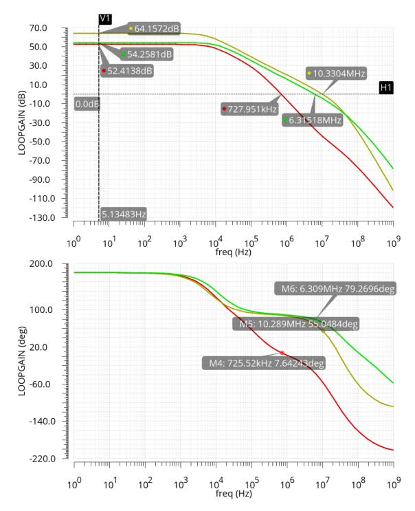
Figure 4.1: Frequency response for output load current at 0 A, 1 mA and 100 mA
