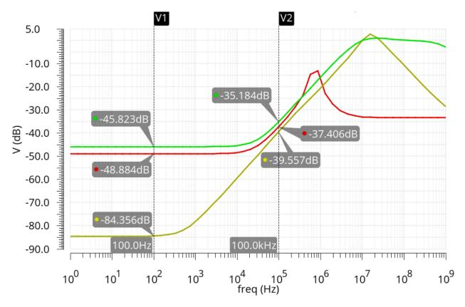
Figure 4.4: PSRR at 0, 1 mA and 100 mA load current
