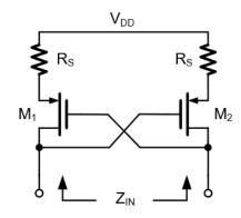
Figure 3.10: Cross-coupled pair with source degeneration resistors
