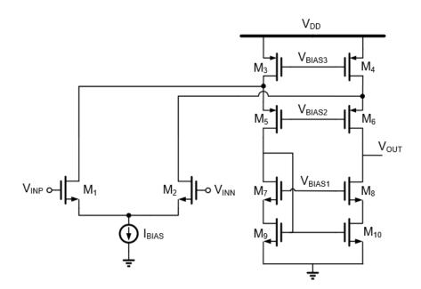
Figure 3.7: Low voltage folded-cascode OTA
