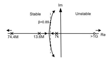
Figure 3.30: Root locus for 1 mA load
