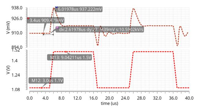
Figure 4.7: Line transient response at no load
