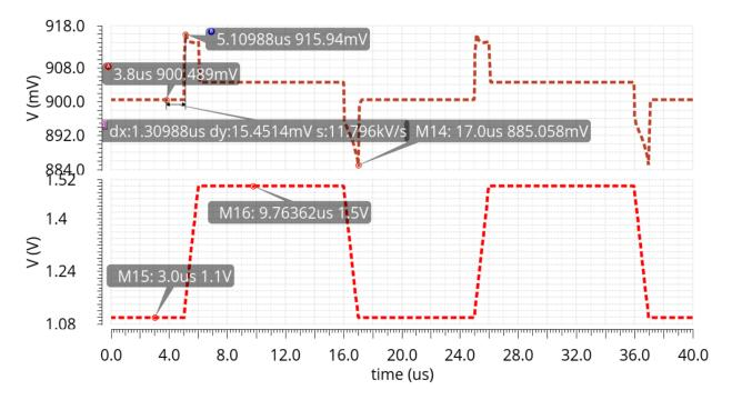
Figure 4.8: Line transient response at 100 mA load
