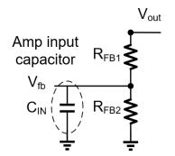
Figure 3.19: Parasitic capacitor in feedback network
