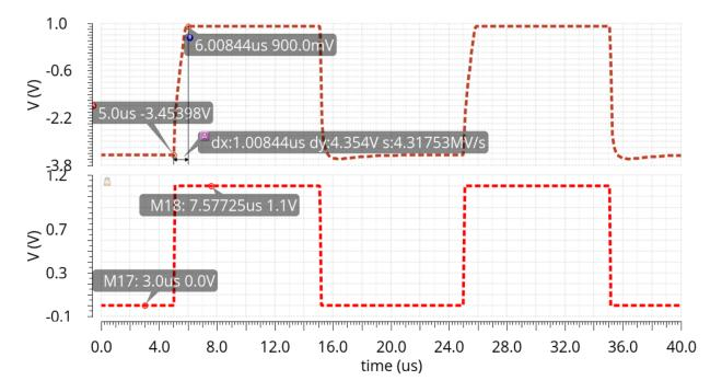
Figure 4.10: Start up condition with 100 mA load current
