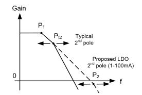
Figure 3.24: Capacitor-less LDO output pole movement
