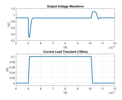
Figure 3.13: Uncompensated transient response
