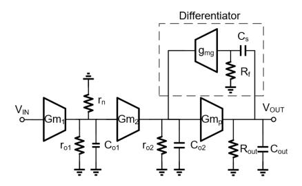
Figure 3.34: Small signal model of the proposed LDO during transients
