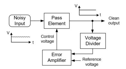
Figure 1.4: Typical block diagram of a linear regulator
