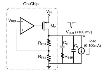
Figure 2.6: Macro model of the uncompensated load transient
