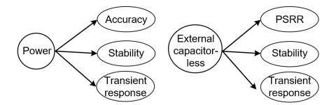
Figure 3.1: Low power external capacitor-less design trade-offs
