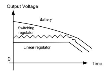
Figure 1.2: Output voltage after battery and different regulator
