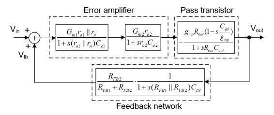
Figure 3.21: Block diagram of the proposed LDO
