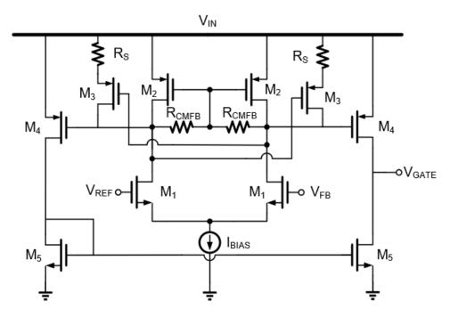
Figure 3.12: Two-stage gain compensated error amplifier
