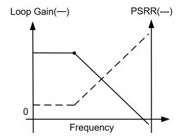
Figure 2.5: PSRR with frequency
