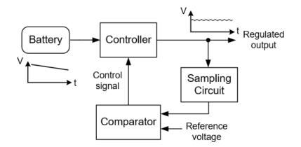
Figure 1.3: Typical block diagram of a switching regulator
