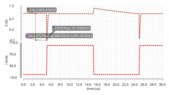
Figure 4.5: Uncompensated load transient response
