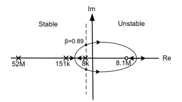
Figure 3.28: Root locus for sweeping feedback factor at no load
