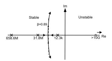
Figure 3.32: Root locus for sweeping feedback factor at 100 mA load
