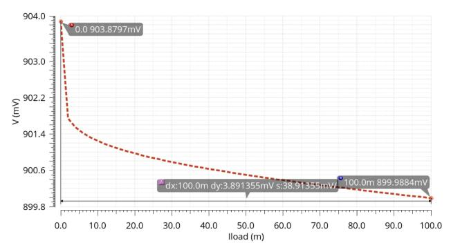
Figure 4.2: Load regulation with load from 0 A to 100 mA
