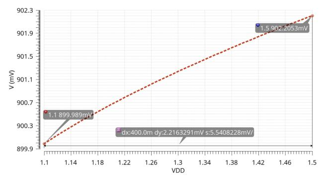
Figure 4.3: Line regulation at 0 A load current
