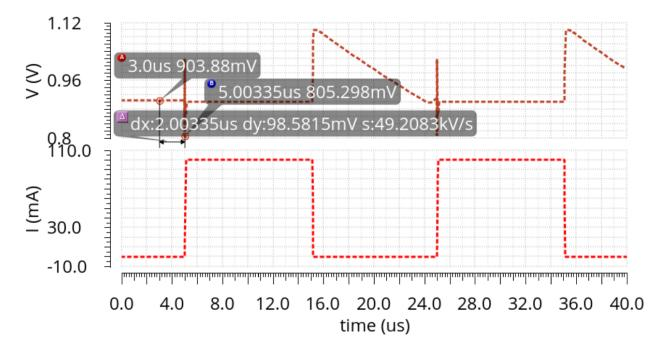
Figure 4.6: Compensated load transient response
