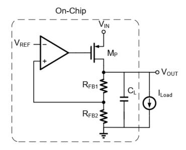
Figure 2.9: External Capacitor-less LDO
