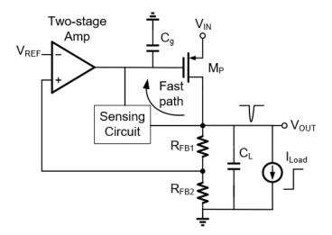
Figure 3.14: Transient-enhanced circuit concept
