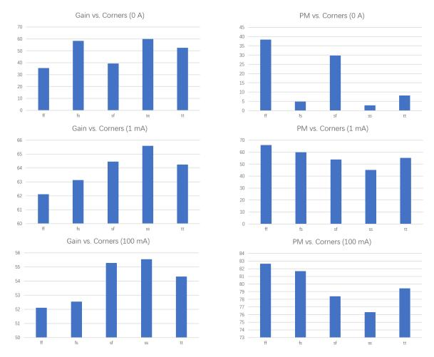
Figure 4.17: Loop gain and phase margin for 5 corners at 0A, 1mA and 100mA
