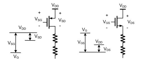
Figure 3.4: Input swing comparison between NMOS and PMOS pass transistors
