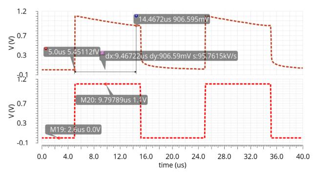
Figure 4.9: Start up condition with 0 A load current
