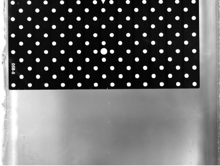
Figure 4.8: Calibration plate image at plane B used in determination of  $M$  for the first test. Similar images were collected for the second test.
