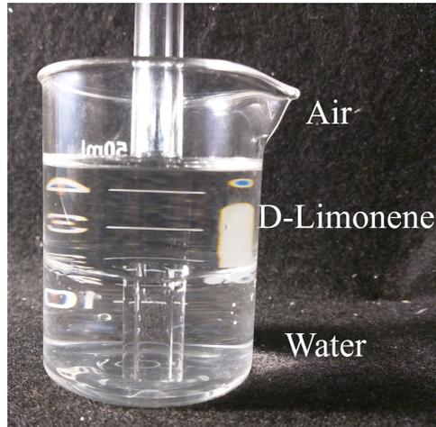
Figure 3.1: Borosilicate glass tube submerged in a non-mixed combination of D-limonene and water. Lack of light ray refraction can be observed via the horizontal lines on the glass container, which are partially behind the submerged tube.
