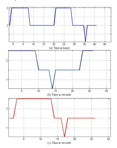
**Figure 9.** (a) Consumption pattern (CP) predicted states; (b) tap event (TE) predicted states and (c) seepage event (SE) predicted states against 300 future points (hours for (a) and seconds for (b) and (c)) from HHMM.
