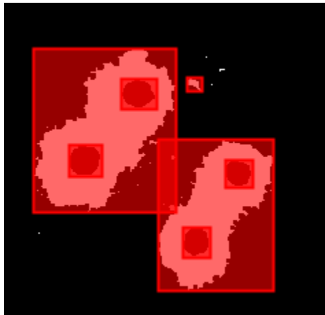
Figure 1.3: Antenna recognition system failure caused by overlapping boxes
