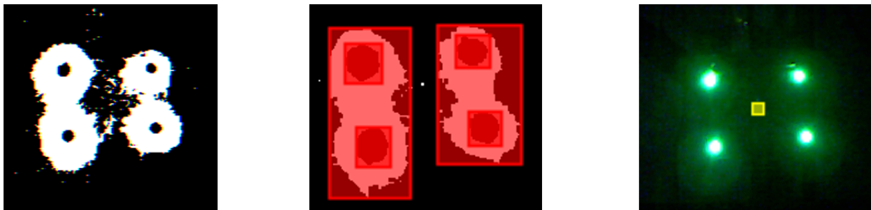
Figure 1.2: Computer Vision System: (left to right) Patch Antenna with LEDs Filtered, Boxes Drawn Around Sharp Filtering Contours, Successful Feed Point Location
