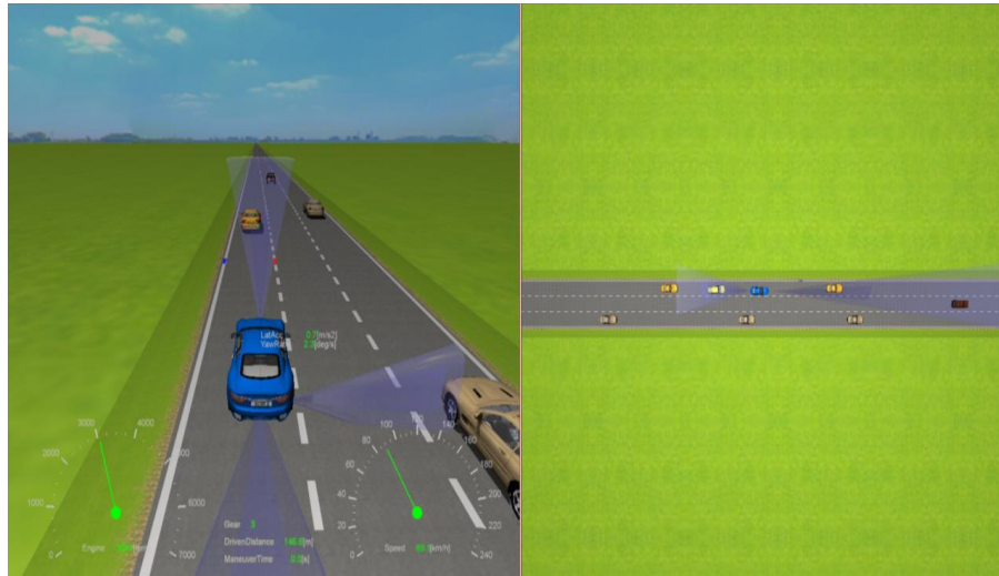
Figure 2.27: SV turns on the turning signal and adjusts its speed in order to merge the gap ahead of TV2 . Even though TV2 's objective is to prevent SV from lane changing, SV seeks to maximize the lower bound of TV2 's action
