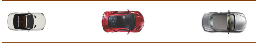
Figure 1.8: A car following model in highway driving. The subject car is in the middle, and the front vehicle is the lead car. The subject vehicle reacts to the change in the speed of the lead car. The rear car also reacts to the speed change of the subject car.
