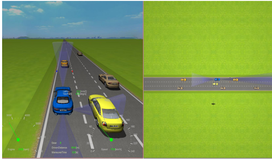
Figure 2.26: This graph is intended to show the visual set-up, with two different camera orientations of the simulated traffic. First, the SV starts with an initial speed of 22\text{ m/s} and it encounters an obstruction in its drive lane and searches for a gap.
