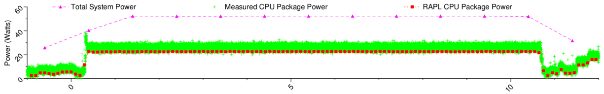
Figure 5.1: Comparison of RAPL values vs. Measured values [8]
