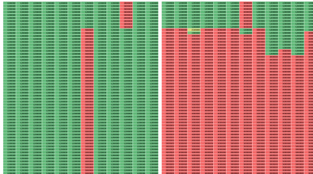
Figure 4.2: Core Frequencies running blackscholes using (3.5) (left) and (4.3) (right)
