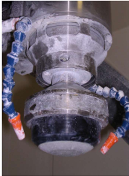
Figure 13: Photograph showing the Bonnet polishing flexible head mounted on CNC (Reprinted from [27])
