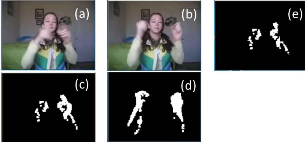
Figure 4: Generation of speed frames. (a) Previous frame (b) Current frame (c) Foreground image of (a). (d) Foreground image of the (b) (e) The speed frame generated using (c) and (d)
