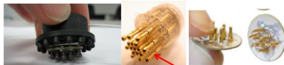
Figure 1.1 - Finger based dry electrodes. Individual images taken from (left to right) [19-21]. Reprinted from Design Principles and Dynamic Front End Reconfiguration for Low Noise EEG Acquisition with Finger Based Dry Electrodes, Viswam Nathan and Roozbeh Jafari, IEEE Transactions on Biomedical Circuits and Systems, ©2015, IEEE
