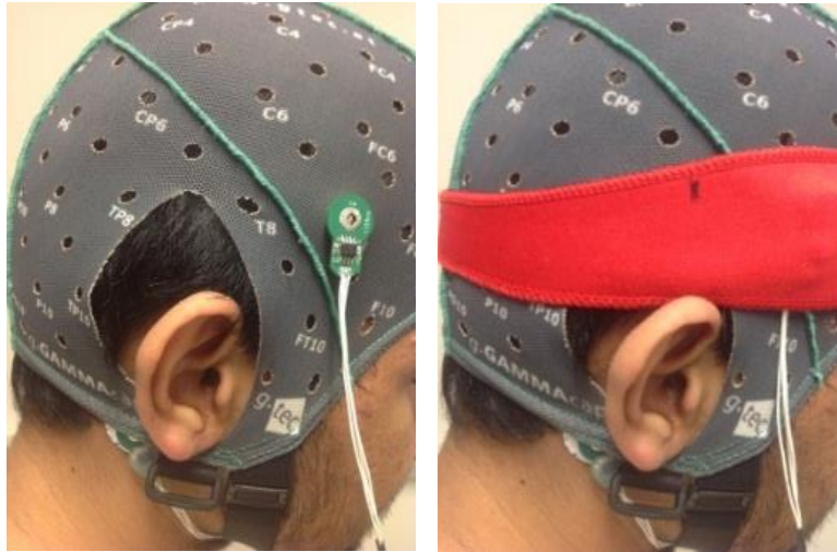
Figure 4.4 – Impedance measurement at FT8 without headband (left) and with headband (right). Reprinted from Design Principles and Dynamic Front End Reconfiguration for Low Noise EEG Acquisition with Finger Based Dry Electrodes, Viswam Nathan and Roozbeh Jafari, IEEE Transactions on Biomedical Circuits and Systems, ©2015, IEEE
