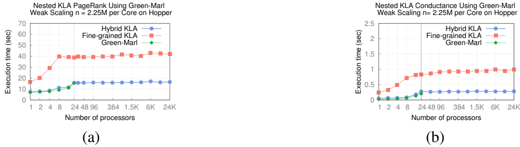
Figure 8.10: Nested KLA with Green-Marl for (a) PageRank and (b) conductance, up to 24,000 cores.
