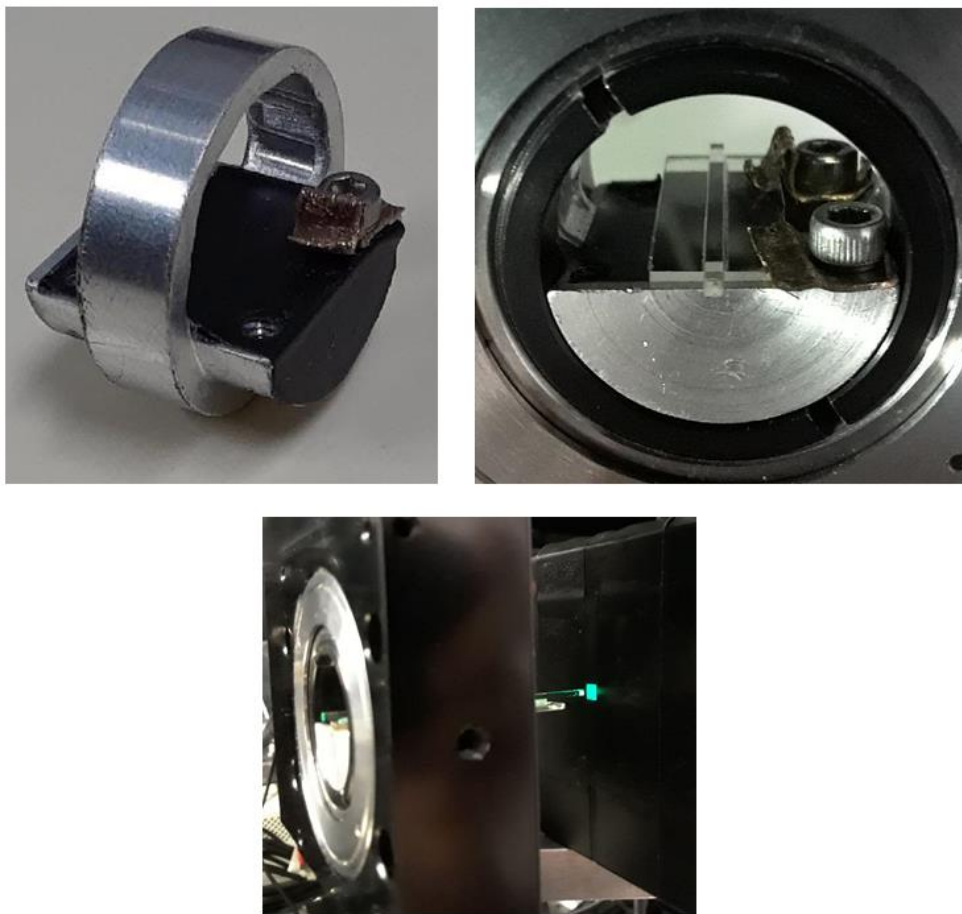
Figure 42 Rotation mount insert (top left) providing \phi adjustment ability. Sample LP on mount in place within rotation stage (top right). 50 mm x 1 mm x 1 mm LP testing in situ (though translated out of the detector for the image) using insert and stage (bottom).
