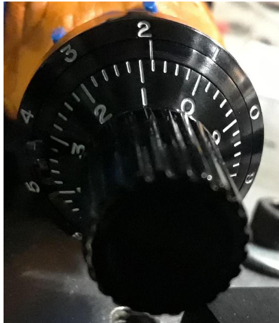
Figure 76 Counting dial/knob used with the theta rotation stage.
