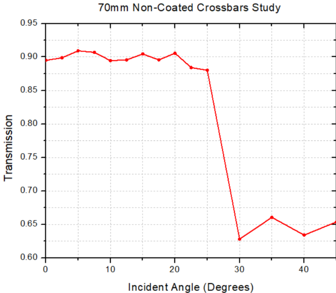
Figure 52 Scan interrogating original sides where one is mounted at two locations to non-coated crossbar supports through the use of a n = 1.328 adhesive.
