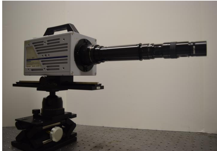
Fig. 4.6 Photron SA3 high speed camera utilized to capture droplet images
