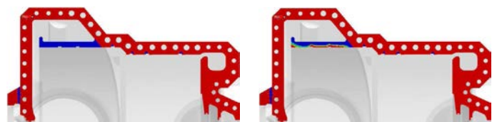
Figure 26. Gap at flange for optimized casing with applied test pressure (left) and pressure + temperature in operation (right).
