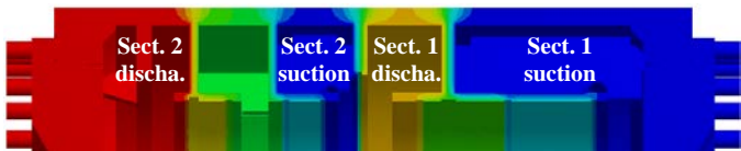
Figure 15. Temperature distribution in operation (steady state).
