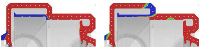
Figure 24. Gap at flange for draft casing with applied test pressure (left) and pressure + temperature in operation (right).
