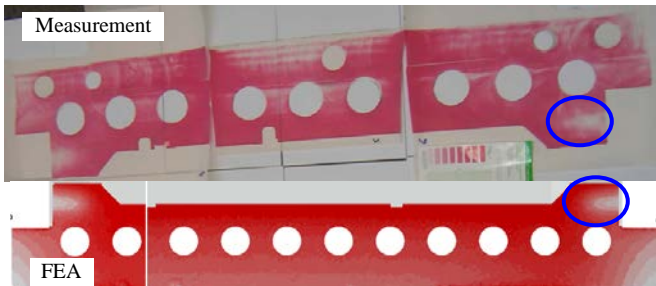
Figure 8. Pressure distribution after pretension (FEA and Film).
