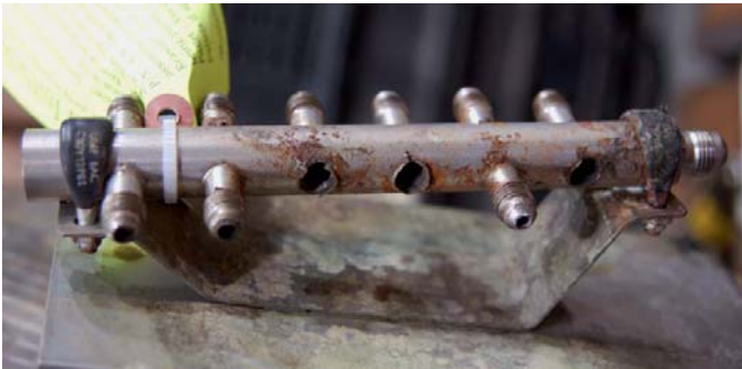
Figure 2. Liquid Fuel Flow Divider Aqueous Corrosion
