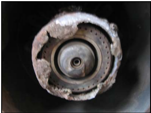
Figure 3. Fuel Injector Tip Sulfidation
