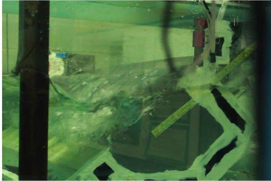
Figure 35. Vortex and Bubble at the Ramp
