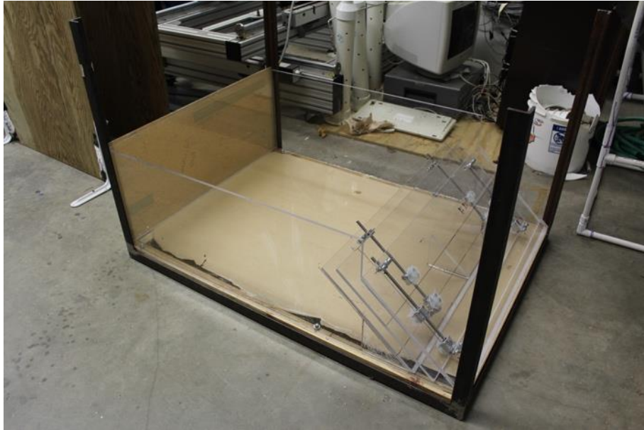
Figure 12. Scaled Overtopping Structure Model
