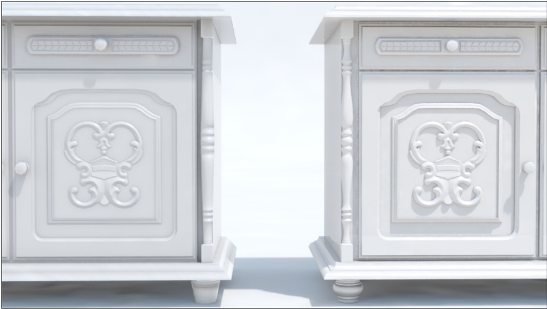
Figure 5.11. Normal texture baking facilitates the transference of surface qualities from high-poly models (right) to low-poly models (left).
