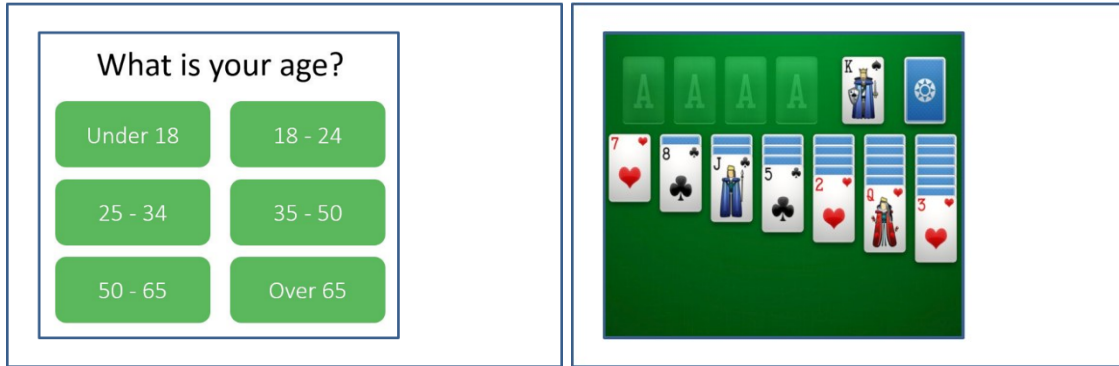
Figure 5. Two examples of the gesture interaction system’s visual interface, with different interactive applications: a questionnaire and a card game. The application area is nested within the display and it may contain any application interface that supports simple touchscreen-like interaction. The area surrounding the application interface is dedicated for affordances and feedback of the gesture interface.
