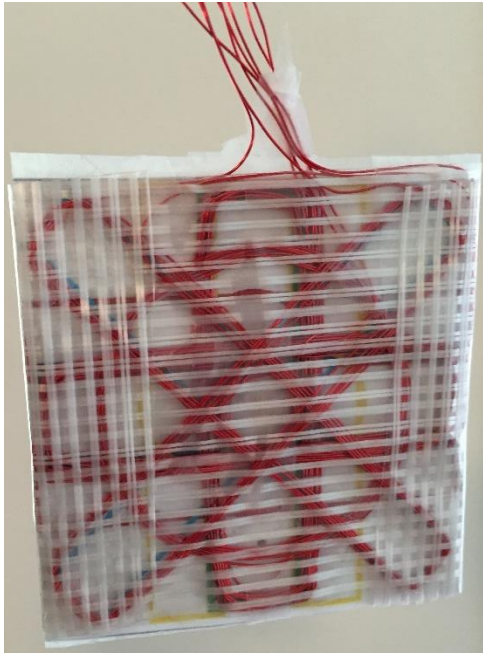
Fig. 12: One side of shim coil setup.
