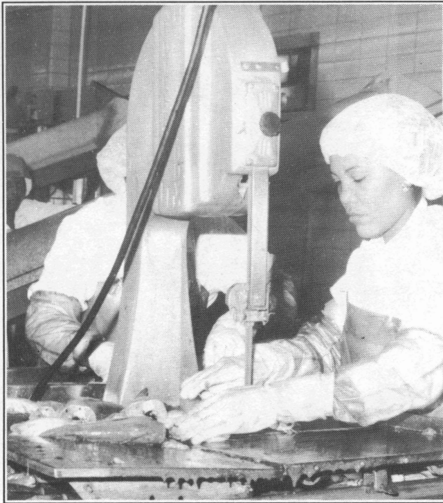
Figure 3. Deheading channel catfish with a band saw.
