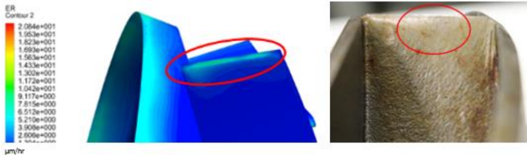
Figure 18: Erosion prediction on pressure side of outer blade
