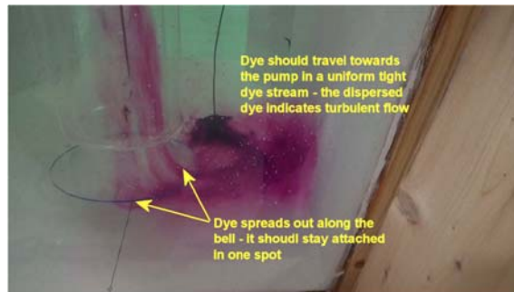
Photo 5-1 Unsteady Flow Around the Pump
