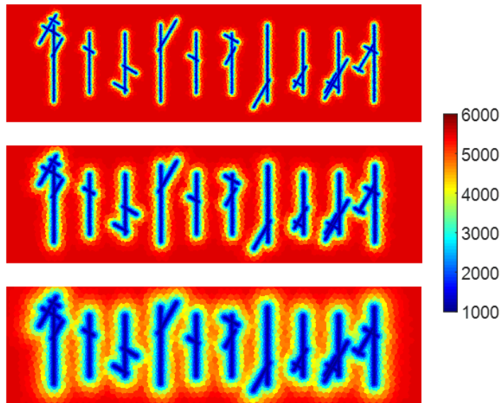
Figure 3.27 Pressure distribution for 2D multiple fracture model: a) 3 months; b) 1 year; c) 3 years
