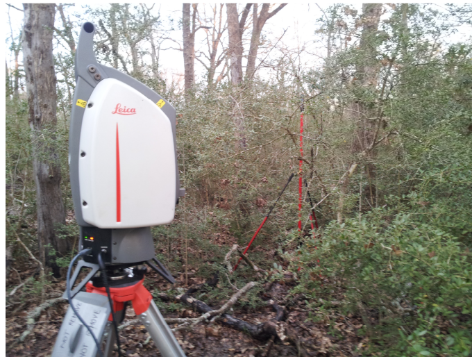
Figure 2: Leica ScanStation 2 terrestrial laser scanner and flat scanning target at site 1.
