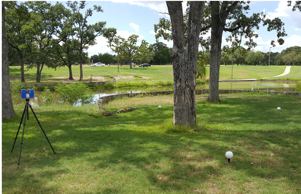
Figure 3: FARO Focus 3D X 330 terrestrial laser scanner and spherical scanning targets at site 3.
