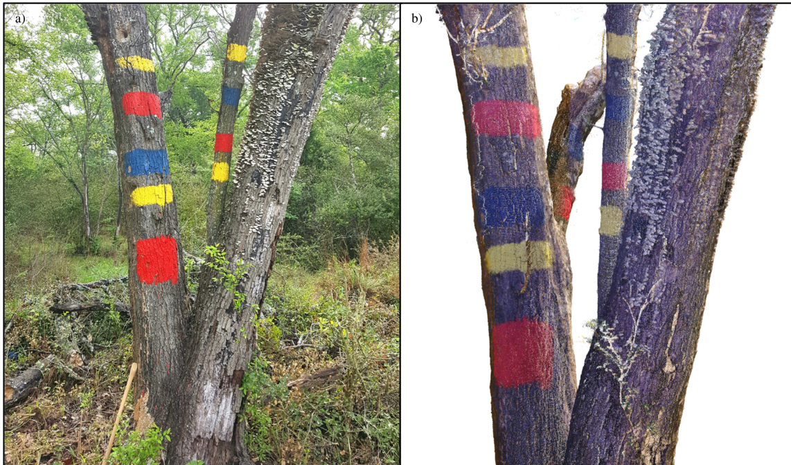
Figure 12: Q. stellata SDT (a) and colored point cloud (b) with painted stem and branch sections used to identify and extract the accuracy assessment samples in the processed voxel model after the tree was felled and sectioned.
