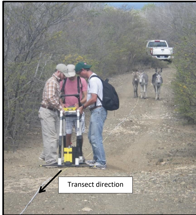
Figure 6: Common-offset acquisition. Showing two individuals (left and right) moving the equipment along a transect with another (center) operating the transmitter trigger and data logger, (foreground). Black arrow indicating transect direction.
