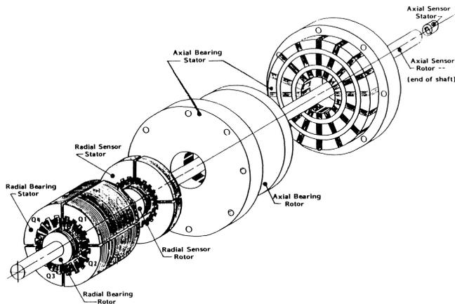
Figure 1. Radial and Axial Bearing Configuration.
