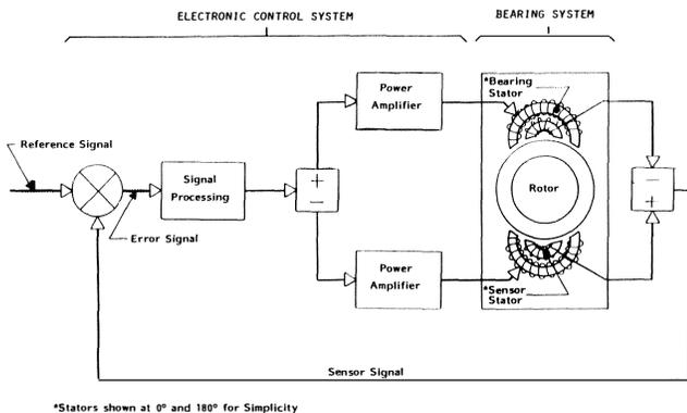
Figure 2. Basic Control Loop Diagram.
