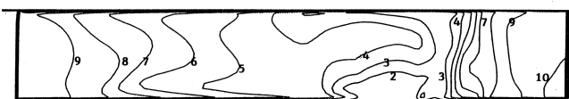
Figure 16. Controlled Inlet Pad Cavity Radial Mid Plane Temperature Distribution for Laminar Flow.
