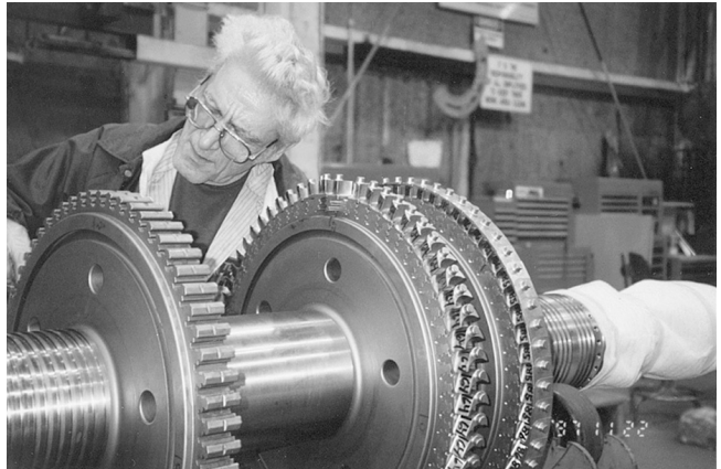
Figure 22. Loading Buckets into Turbine Rotor Wheels.
