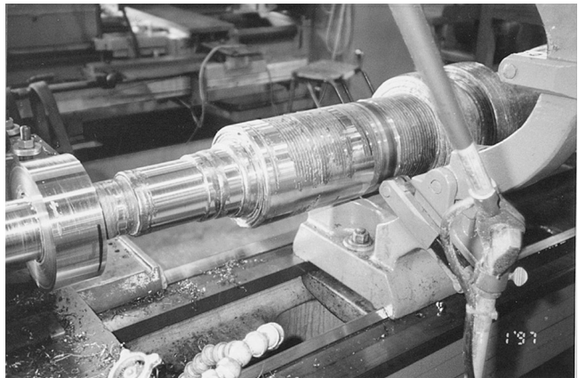
Figure 17. Machining after Initial Weld Pass.
